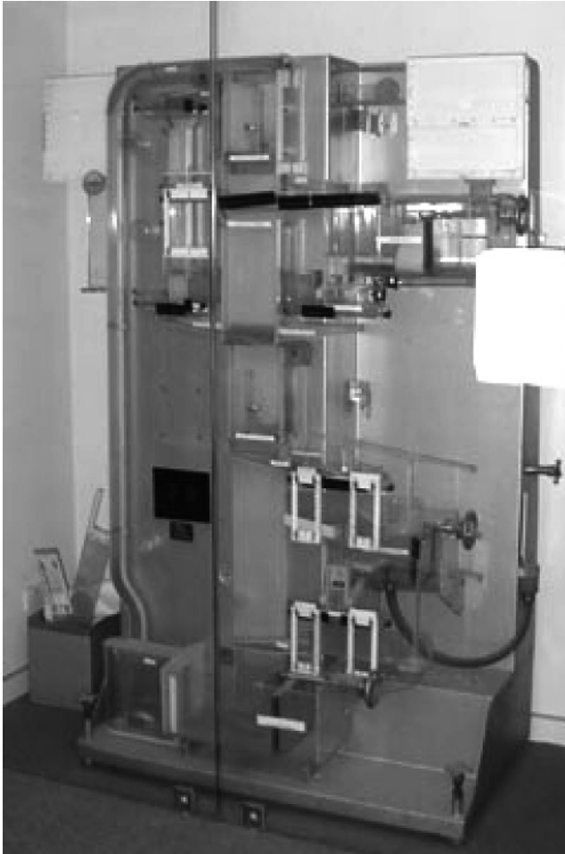
Figure 1.1 The economy machine. A reconstruction of the Moniac (at the University of Melbourne), a hydraulic simulator of a national economy built in 1949 by A.W.H. Phillips of the London School of Economics, that used the flow of colored water to represent the flow
