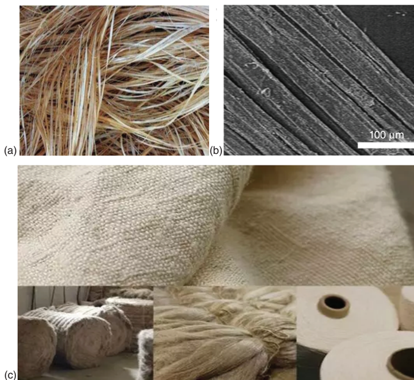
Figure 1.2 Hemp fibers. (a) Photographs of hemp fibers. (b) The SEM of hemp fibers. Source: Mwaikambo and Ansell [2]. (c) Photographs of spinning ropes and sacks for packaging.
