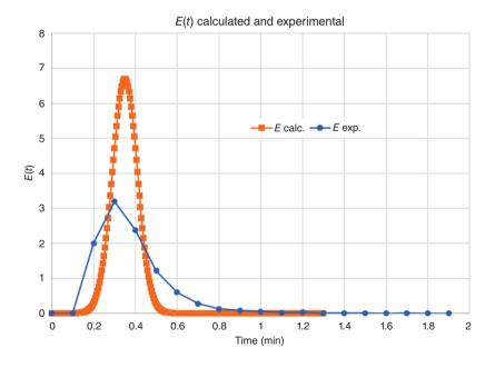
**Problem 1.21** A common issue encountered in the development of gas and liquid phase chromatographic analysis methods is the phenomenon of "tailing." Tailing makes it challenging to characterize the retention time of a specific species due to the prolonged tail associated with the peak. An approximate representation of tailing
