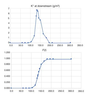
Problem 1.23 By injecting brine into an experimental continuous reactor, a signal is obtained at the exit given by:
