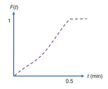
**Problem 1.20** A commercial-scale distillation tray is being studied for residence time using a fiber optic technique. A pulse of a 10 g/l solution of Rhodamine-B dye was injected into the downcomer of the top tray. The response data, summarizing the time (min) and corresponding output voltage (V), are provided as follows:
