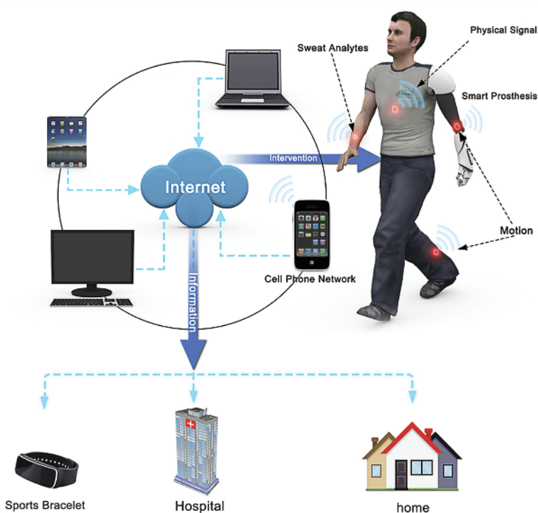
Figure 1.4 Conceptual diagram of the application of wearable electronics in smart sensing technologies, human-machine interfaces and health monitoring, interconnecting daily activities with facilities, devices, and mobile terminals. Source: [12]/John Wiley & Sons/CC BY 4.0.
