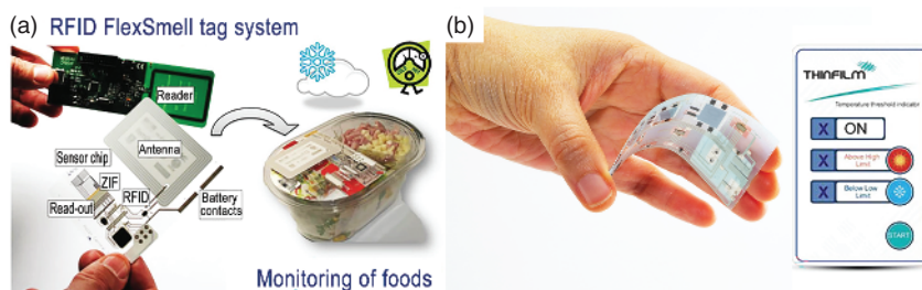
Figure 1.5 Smart tag for monitoring of foods. (a) Inkjet-printed multisensory platform. (b) A smart temperature-sensing label consisting of memory, display, and wireless communication unit. Source: [26]/with permission of John Wiley & Sons.
